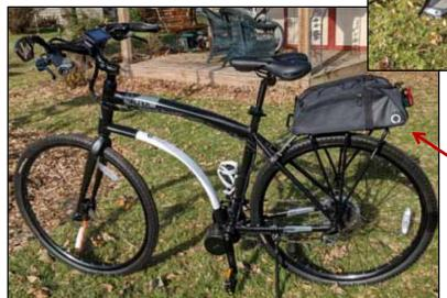
Battery is hidden in rear trunk (an available option on any build).
