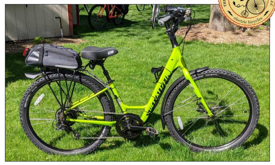
A customer's Specialized Roll Sport bike upgraded to electric assist with optional rack, bag, fenders, grips seat and more. Upgraded with a 1 hp, 750 watt nearly silent motor mid-mounted (standard on all builds). Battery discretely located behind seat.
